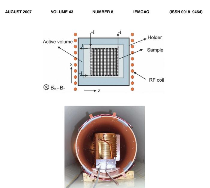
Sample holder (above) and radio-frequency coil located in the magnetic field of a magnetic resonance imager (below) used to image magnetic field distributions in thin layers of biological and physical samples. See "Indirect Susceptibility Mapping of Thin-Layer Samples Using Nuclear Magnetic Resonance Imaging" by I. Frollo, P. Andris, J. Přibil, and V. Juráš on page 3363.
