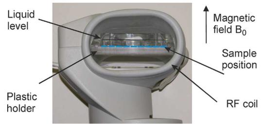
Fig. 7. Horizontal field hand/wrist RF coil and plastic holder (homogeneous phantom), active circular diameter 90 mm.
