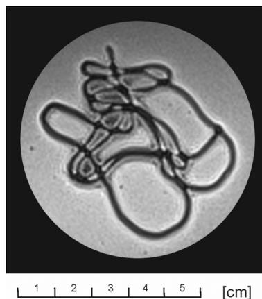
Fig. 12. MR image of the polymer fiber, thickness 0.14 mm, treated by the water solution of  $\text{Fe}_3\text{O}_4$  nanoparticles. Number of measured samples, measured matrix:  $256 \times 256$ . Actual image of this sample was associated with  $100 \times 100$  pixels.
